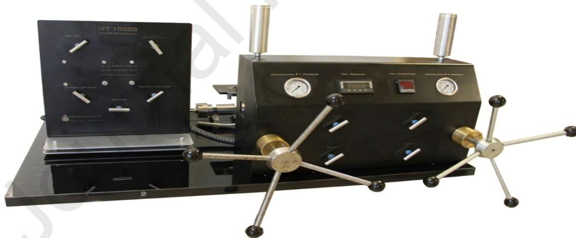
258 **Fig. 2.** Apparatus and schematic of the high-pressure/high-temperature IFT utilized in this study
